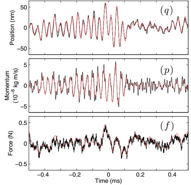
FIG. 2 (color online). Time-domain results for (q) position, (p) momentum, and (f) external force, respectively, with  $|\alpha|^2 = 6.24 \times 10^6$  s<sup>-1</sup> and the probe beam in a phase-squeezed state. The black lines are the signals to be estimated. The red lines (gray lines in print) are the estimates.
